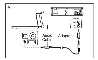
B. Plug one end of the audio cable into the jack on the front of the treadmill near the power cord. Plug the other end of the cable into the included adapter. Plug the adapter into an RCA Y-adapter (available at electronics stores). Next, remove the wire that is currently plugged into the AUDIO OUT jack on your VCR and plug the wire into the unused side of the Y-adapter. Plug the Y-adapter into the AUDIO OUT jack on your VCR.
